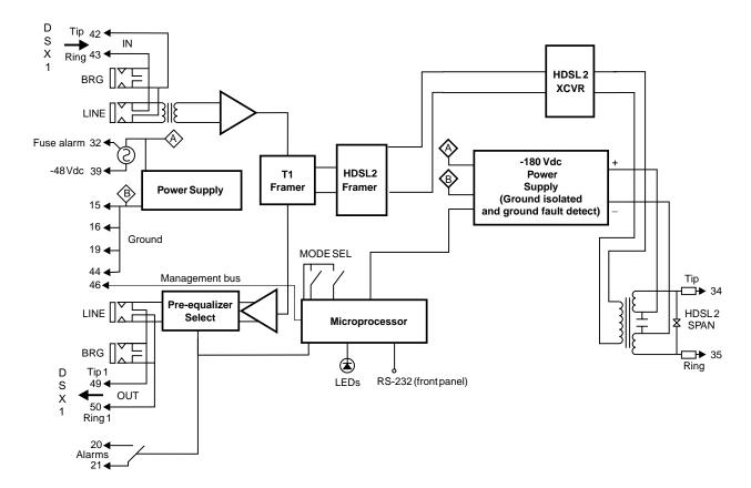
Figure 33. H2TU-C-231 List 2 Block Diagram
